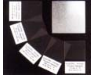
Calibration foil with thicknesses ranging from 10µm up to 15mm
